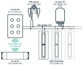
**101 mode** is enabled after a 101 power supply has been connected to the DALI terminal and the device **has not** been added to a 104 application controller.
